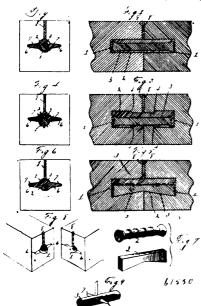
in and crossing the joining-surfaces. 6th. A bond for joining and bracing bodies consisting of a solid bar, and a bar formed around it having circumferential arms, both bars and arms engaging the joined parts.
