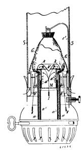
draught in order to produce a gas air mixture, which produces in combination of a sufficient air draught outside the chamber M, a Bunsen flame suitable for incandescent lighting or heating purposes.
