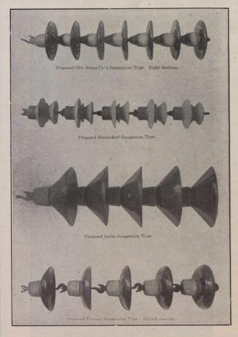
In addition to the electrical tests, the mechanical features of the different insulators were thoroughly investigated. A great number of breaking tests were performed to ascertain the strength and rigidity of the insulators and their connections.
