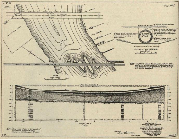
in diameter. / Figure 1 shows the general plan of the Hackensack River at the point where the line crosses; a cross section of the pipe in place in the river bottom; and a longitudinal cross section showing the general character of the supporting soil.
