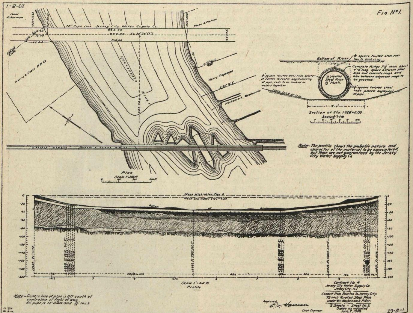
in diameter. Figure 1 shows the general plan of the Hackensack River at the point where the line crosses; a cross section of the pipe in place in the river bottom; and a longitudinal cross section showing the general character of the supporting soil.
