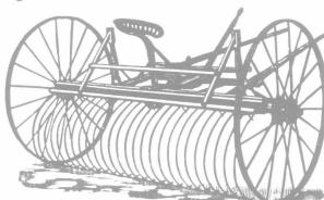
This rake is made with steel wheels. It has 26 teeth, and where the eeth are fastened angle steel is used. The shafts on our rakes are so constructed that they may be used for either one or two horses, if
