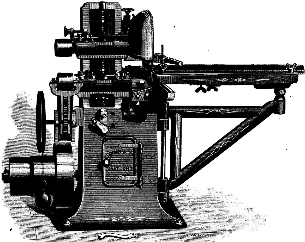
This is an entirely new style of Tenon Machine. The frame is cast in one piece, and the working parts stand solidly on a pedestal, avoiding all vibration.
