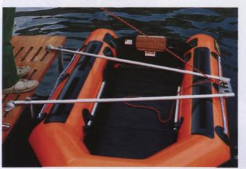
The Dingybat davit system — the simplest, safest method of securing a dinghy.
