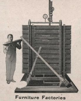
find this a necessary machine because it saves loss due to gluing up moist veneer; and because it makes usuable veneer out of what would otherwise be wasted.
