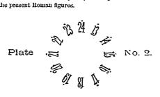
"Plate No. 2 shows the secondary dial. It must be of thin material; and it has been " found that made simply of paper and secured to its position by any gum which will adhere to " an enamelled surface, the object is attained without any further alteration of the watch or • " clock.
