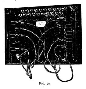
In Electric Light Switch-Boards, or Distributing Switches, spring-jack contacts are connected with the terminals of different circuits, and plug-switches with the dynamo terminals. By these means, any dynamo can be connected with any circuit, or a number of circuits can be connected with the same dynamo, or a number of separate dynamos can be placed in the same circuit, without interference with the lights.
