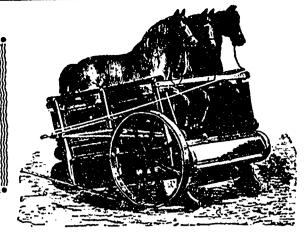
E provide a special brake with our three horse tread power, as stopping the machine suddenly with ordinary brake is apt to force the band wheel.
