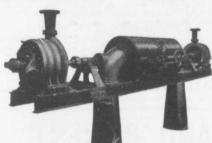
Two Worthington 3-Stage Turbine and McCormack Water Wireels, built for Port Arthur, Ont., Water Works, 1440 gal. per minute against 350 ft. head.
