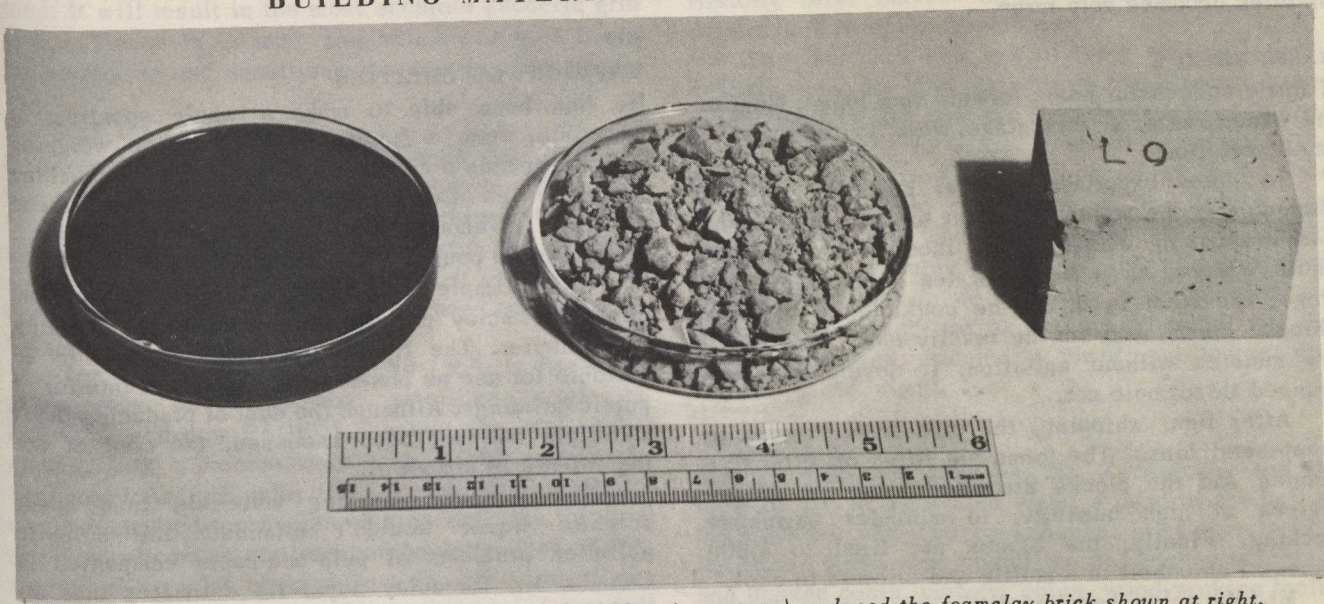
Spent sulphite liquid (left) and common clay (with foaming agents) produced the foamclay brick shown at right.
