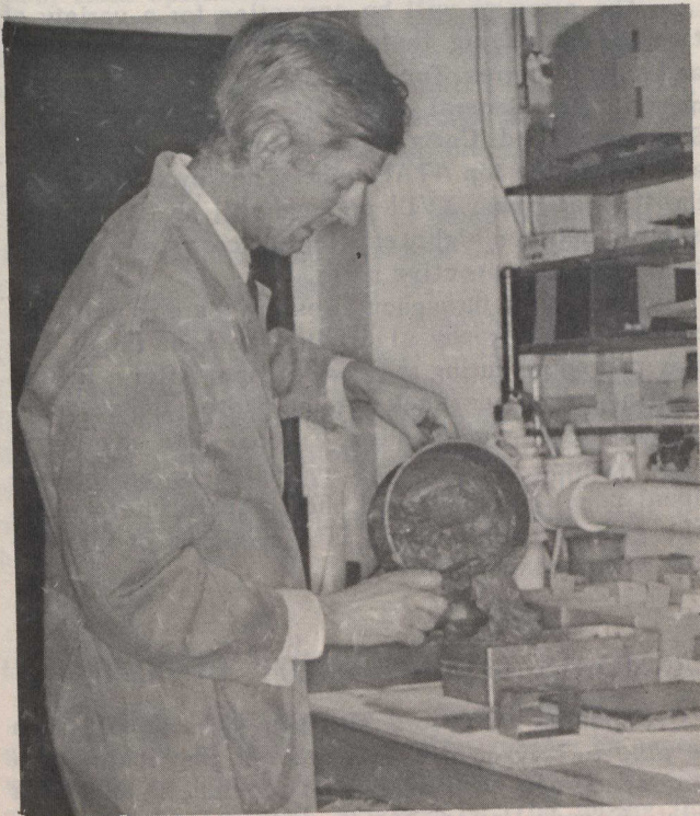
Gavin Macaulay pours a mixture of clay and spent sulphite liquor into a metal mould - one of the final steps in producing foamclay bricks.
