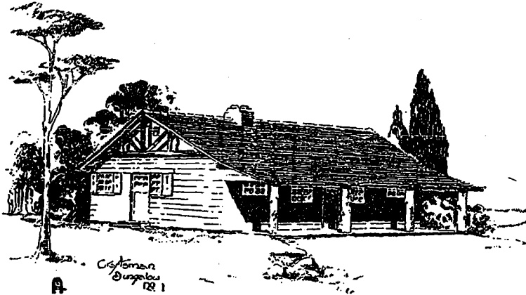
Design No. 7.—A craftsman bungalow, sheathed with boards 8 x 10 inches wide, \frac{3}{4} of an inch thick, laid like clapboards. Note the truss of hewn timber in the gable, which not only forms a decorative feature, but gives added support to the roof.
