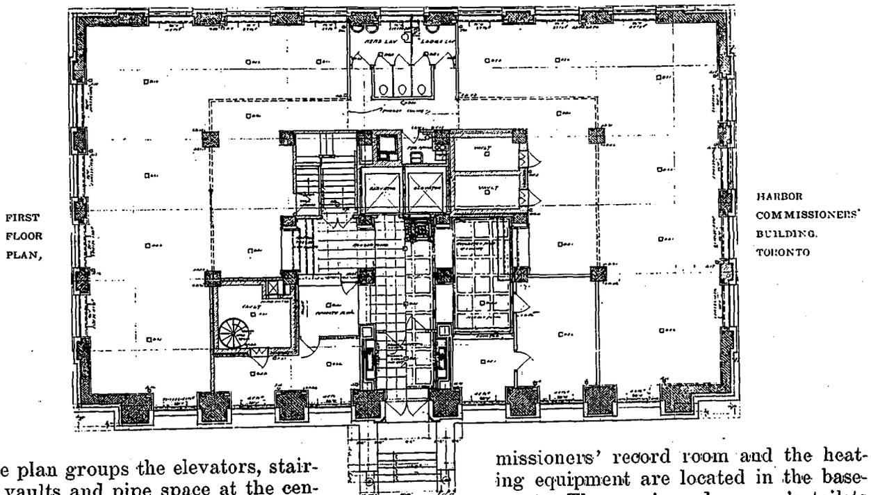
The plan groups the elevators, staircases, vaults and pipe space at the centre with surrounding corridors providing access to offices on four sides. The entrance hall on the first floor is entered from the south front, and has the telephone switchboard
