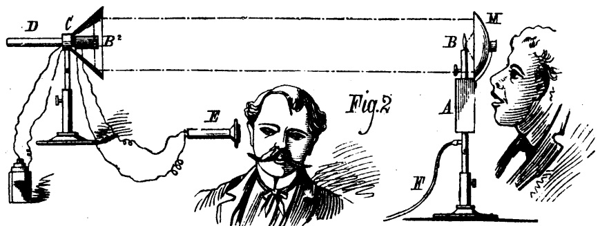
MAGNETIC THERMOPHONE WITH MANOMETRIC FLAME TRANSMITTER.
