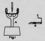
ciently clearly the arrangement of the apparatus. The upper ends of the capillary tubes should be ground to flat discs about 1.7 mm in diameter and coated with paraffin wax. The two halves of the U-tube are connected by a piece of the fine rubber tubing (0.5 mm bore) used for covering spectacle frames. The U-tube is completely filled with water, and while the rubber connection is closed by pressure with a
