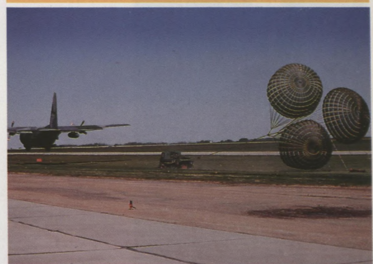
LAPES—Low Altitude Parachute Extraction System, 1.5 m to 3 m (5 ft. to 10 ft.).
