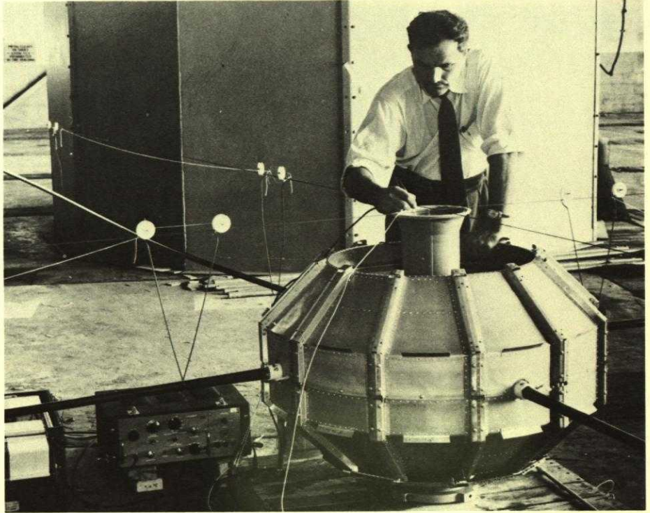
Alouette I, launched in 1962, had two antennas. Each consisted of two poles extended at right angles to one another. Each pole was stored as a tape on a spool (left) during launching. In space, as the tapes unwound, their edges curled tightly together to form semi-rigid tubes. The antennas, shown in tests (right), measured 46 and 23 metres from tip to tip. Later Alouette and ISIS satellites had 73-metre antennas.
