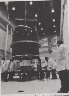
Anik D1 is now undergoing its final integrated system testing at the David Florida Laboratory of the Department of Communications near Ottawa. The \$30-million satellite, which will provide 24 channels at 6/4 gigahertz, is due for launch aboard a U.S. National Aeronautics and Space Administration Delta rocket from Cape Canaveral, Florida next August. Two Anik Ds are being built for Telesat by Canadian prime contractor Spar Aerospace of Toronto.
