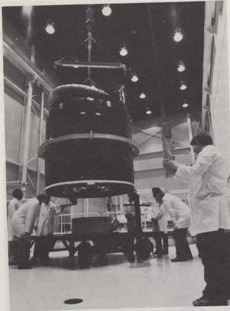
*Anik D1 is now undergoing its final integrated system testing at the David Florida Laboratory of the Department of Communications near Ottawa. The \$30-million satellite, which will provide 24 channels at 6/4 gigahertz, is due for launch aboard a U.S. National Aeronautics and Space Administration Delta rocket from Cape Canaveral, Florida next August. Two Anik Ds are being built for Telesat by Canadian prime contractor Spar Aerospace of Toronto.*
