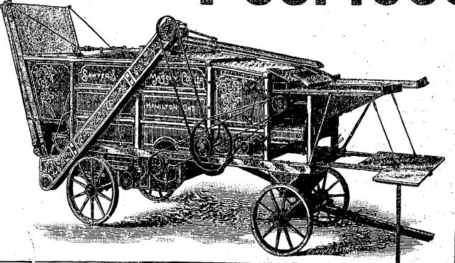
Belt Side View of the "Peerless" Thresher, showing Elevator and Straw Stacker folded.
