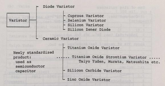
As shown in the chart above, varistors are classified into diode varistors and ceramic varistors. Due to their excellent surge current absorptiveness, production of ceramic varistors is swelling to stand abreast of diode varistors in their volume on the market.
