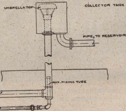
AT THE LEFT,—AIR LIFT PUMP; ABOVE,—TYPICAL ARRANGEMENT OF AIR-LIFT, INCLUDING PUMP, BOOSTER, ELEVATED TANK AND COMPOUND LIFT
