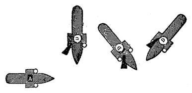
If A secs a White Mast-head Light above the Green Light, A knows that the vessel is a steam-vessel, and is either approaching her in the same direction as B, or is crossing to starboard in some direction, as DDD.
