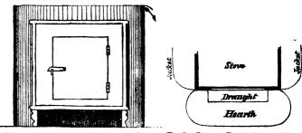
Fig. 4.—ELEVATION OF FRONT PART OF STOVE, Fig. 5.—PLAN OF FRONT PART OF STOVE, SHOWING FITTING OF JACKNT. SHOWING FITTING OF JACKET.
