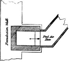
Fig. 2. -PLAN AT BOTTOM OF VENTILATING SHAFT.
