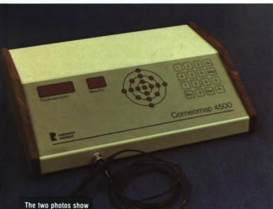
Ine two photos snow an occulometer device for taking internal eye measurements; and a corneomap for mapping cornea of the eye. Both are manufactured by Radionics Medical Inc. of Scarborough, Ontario. remove the secondary cataract. It does so by passing through the artificial lens of the eye without damaging it.
