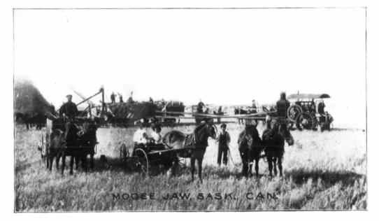
THE HART-PARR is built for power. Every detail of its construction is made to serve that end. It is rated considerably lower than the actual horse power developed; hence there is always an abundance of power in the belt and at the draw bar. Considered as a threshing engine its superiority over the steam tractor is at once apparent. Being oil-cooled it is entirely independent of the water supply, which dispenses with from one to two teams and as many men.
