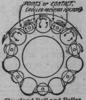
Cleveland Ball and Roller Bearing eeds 35,000 revolutions per minute for months with-
