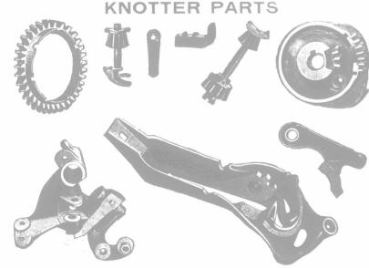
The Massey Harris Knotter is adjustable, so that wear on the pinions may be taken up. Seven sheaves are tied by one revolution of the cord-holder
