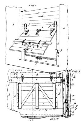
for cars of a pair of eccentrics carried by the car body one on each side of the grain door, substantially as described, and for the purpose set forth. 5th. The combination with a grain door for cars of a pair of eccentrics carried by the car body one on each side of the grain door, and a pair of corner plates, substantially as described and for the purpose set forth.
