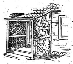
an outside point of view. The cut shows the porch and tells its own story of construction, even to the vines that run up over wire netting on either side and make a charming little arbor within. The curved roof, continuous with the house roof, gives a very pleasing effect to the whole. Such a porch would cost little save the two days' labor of a carpenter.—'N. E. Homestead.'
