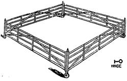
Dimensions-20 feet square, 3½ feet high. Corner Posts 4x4 n. Wheels 8 in. diameter.
