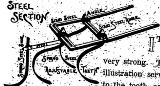
IT is constructed almost entirely of Steel, and is very strong. The Helper shown in the illustration serves as a spring support to the tooth, and prevents it breaking on a sudden recoil.
