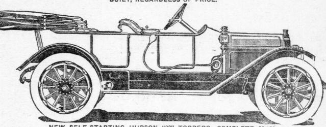
NEW SELF-STARTING HUDSON "33" TORPEDO-COMPLETE, \$2.150. A smart car, short coupled, with long, low, rakish lines and high-back comfortable seats. It is equipped with magneto and storage battery, genuine mohair top, glass windshield, 34 x 4-inch tires on Demountable Rims, extra rim and tire irons. Inside control, full lamp equipment with Prest-O-Lite tank, big beautiful lamps enameled black. Robe and foot rails, cocoa floor mat. Tool box on running board. Tools, license number holders, etc.
