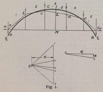
of the compilation of tables and diagrams usually helps to dispel much of the dread. The primary reason of the difficulty in the determination of the stresses in arches arises from the fact that in most cases the arch is what is called "a statically indeterminate structure," so that the forces acting upon the arch cannot be found by the ordinary laws of statics. Exactly similar difficulties arise in the case of stiffened suspension bridges, continuous beams, and slabs.
