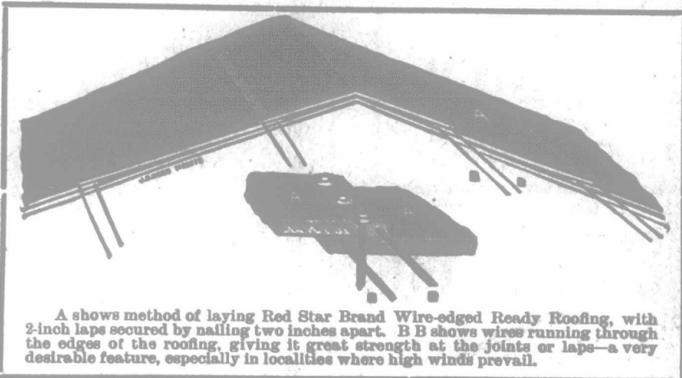
A shows method of laying Red Star Brand Wire-edged Ready Roofing, with 2-inch laps secured by nailing two inches apart. B B shows wires running through the edges of the roofing, giving it great strength at the joints or laps—a very desirable feature, especially in localities where high winds prevail.
