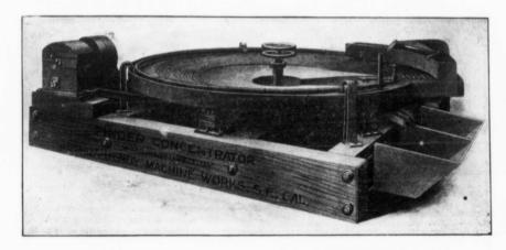
brown linoleum, which experience has proven to be the best substance that can be used for the purpose, and on this surface is laid brass or copper tapering riffles, fifty-six in number, and three-quarters of an inch apart, so arranged as to radiate spirally from the direction of the centre outwardly and around toward the rim, the feather ends terminating in regular sequence nearly in a circle so as to leave a clear smooth space between the terminals and the rim of the pan.
