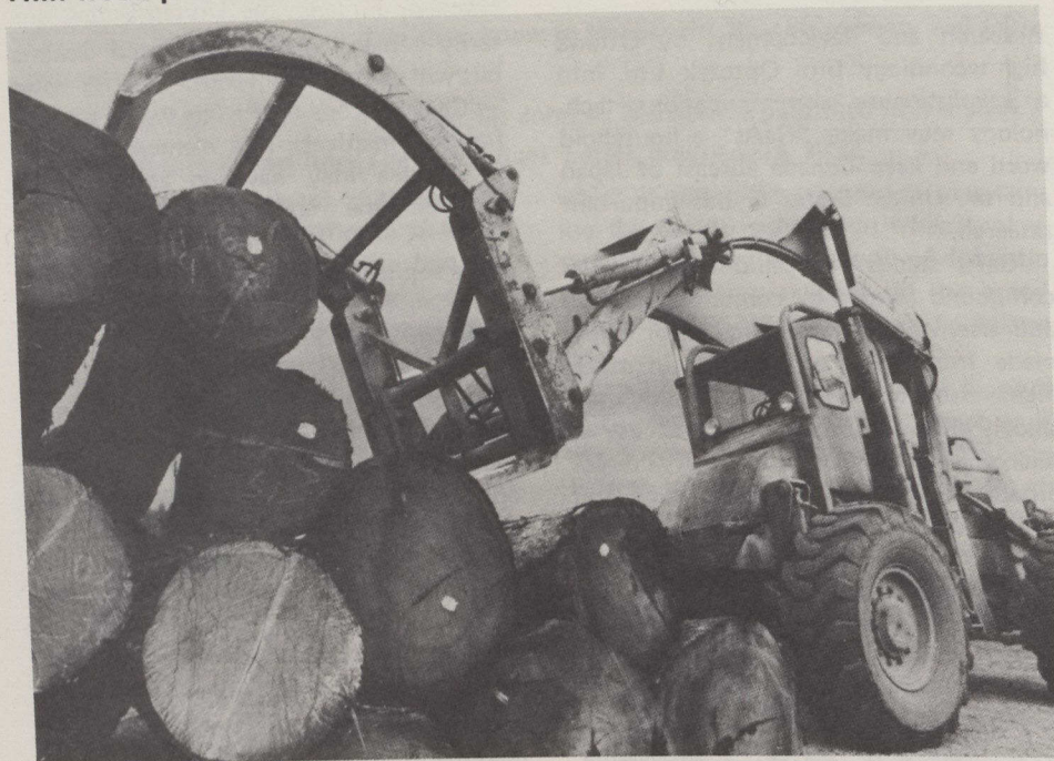
Logs to be processed into veneer are gobbled by a log-loader.
