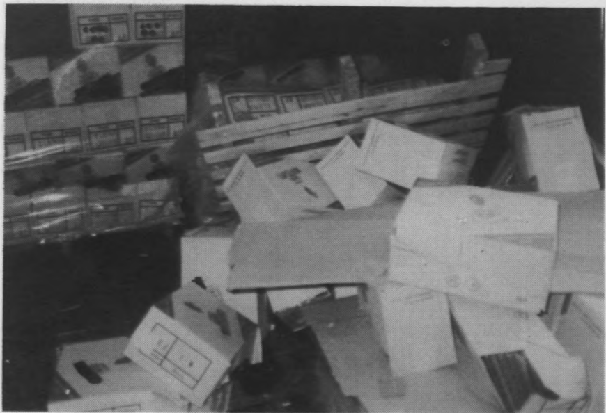
No cargo separations, no proper layering or bracing.
