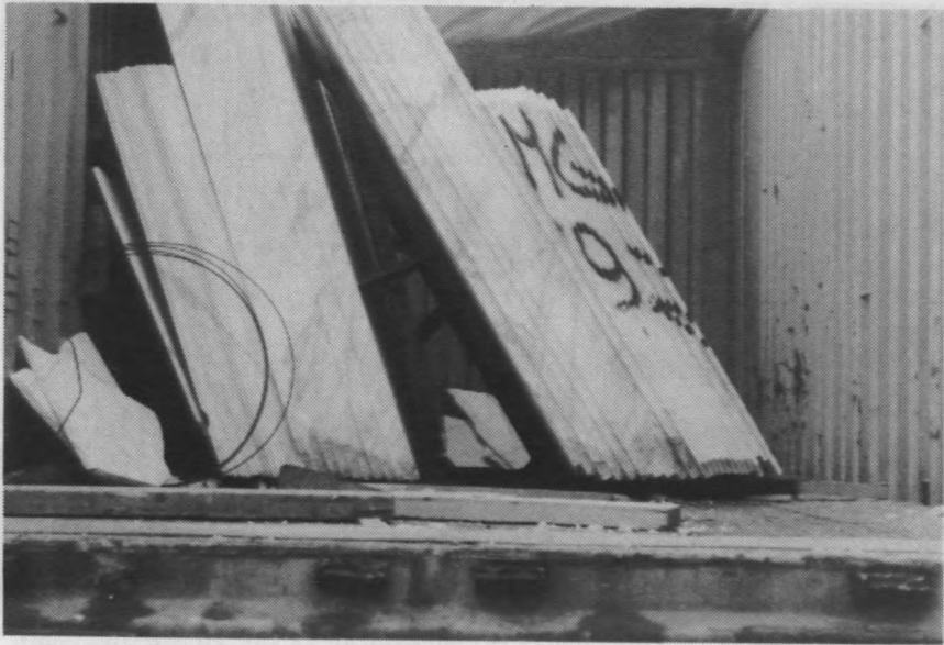
No bracing supports or strapping.
