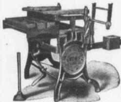
ONE man operating makes 5,000 brick per day. All brick polished on every side with frog impression. This machine uses our Patent Self-racking Pallet, allowing brick to be manufactured where the building is to be erected. Let us tell you all about it. Send for Catalog No. 2. We also make a full line of Concrete Machinery. Tell us your requirements.
