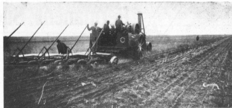
(Note the fine work.) A ten bottom John Deere Engine Gang with a Sawyer Massey Steam Engine (Silver Medal Winner)
