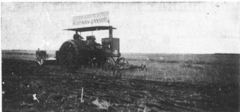
A ten bottom John Deere Engine Gang being pulled by Aultman Taylor Gas Tractor (Gold Medal Winner)
