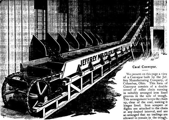
The chains that are used in the construction of these Conveyors, are made with special, large rollers, which materially lessen the power required to drive them, as each link acts as a truck, when running in the iron lined grooves. Coal may be taken into the Conveyor at any point along the line, and may be discharged in like manner, by simply removing suitably arranged slides in the bottom of the trough. For further particulars address manufacturers as above.
