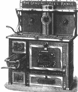
Made of heavy steel plate, braced and riveted removable grate, that can be drawn out and repaired without disturbing the fire linings. Fully tested and guaranteed to take on 25% less fuel than any cast iron range in the market. Send for circular and price list.
