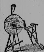
With this Grindstone you can grind all kinds of tool yourself without aid. It runs like a bicycle, you sit down on the seat and work the treadles with both feet. It enables you to do faster and better work than the old way; has self-watering attachment; seat adjustable in height and length, stone can be adjusted on frame.
