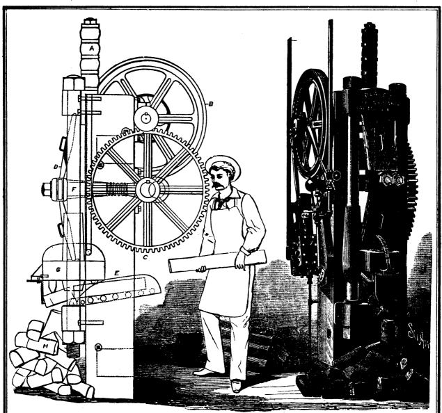
A-Rubber spring for raising the jaws or knives. B-Fly-wheel. O-Gear-wheel. D-Toggie. E-Trough containing pig to be broken. F-Connecting rod for moving toggie. G-Sliding head. H-Iron broken to size.
