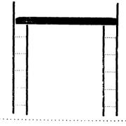
Strips 1 x 3 inches x 2 ft. are nailed across the rows of studding, and at intervals of 2 ft. right up the rows as shown in drawing, beginning within 2 in. or 3 in. of the bottom; this prevents the studs from spreading when the sawdust packing is put in. After all the bents are raised and fastened in position the building is sheeted outside and in, the roof is put on and the walls packed with dry sawdust as also over the joists,
