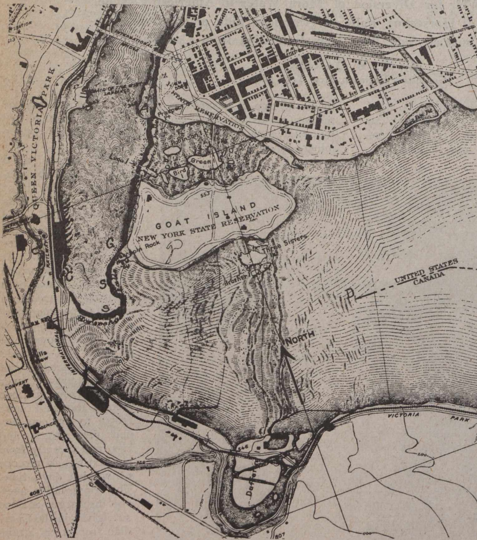
Plan of Niagara Falls, U.S. Geological Survey—A, G and C Indicate Littoral Penstock Installations Proposed by Mr. Young; D, Vertically Controlled Deflector; S, S, Temporary Emergency Main Spillway Section
