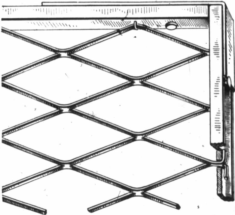
**T**HE ABOVE CUT gives a good idea of Expanded Metal, and shows also how it can be neatly and strongly enclosed in a square frame formed of channel iron for fencing, window guards, and other purposes.
