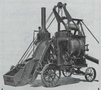
LONDON PAVING MIXER. A forward Loader and rear discharge. No wheelbarrows required. One-third labor saved. The delivery spout is 18 ft. long, swings in a complete circle, distributing the concrete to any part of the roadway. Cuts down the cost. Produces better con-
